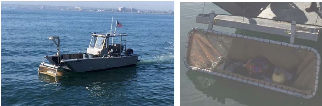
Figure 1. Skimming operations using custom-made hoop net.
